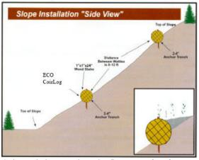
CoirLog helps to reduce the flow rate of surface runoff and collect flowing silt.
